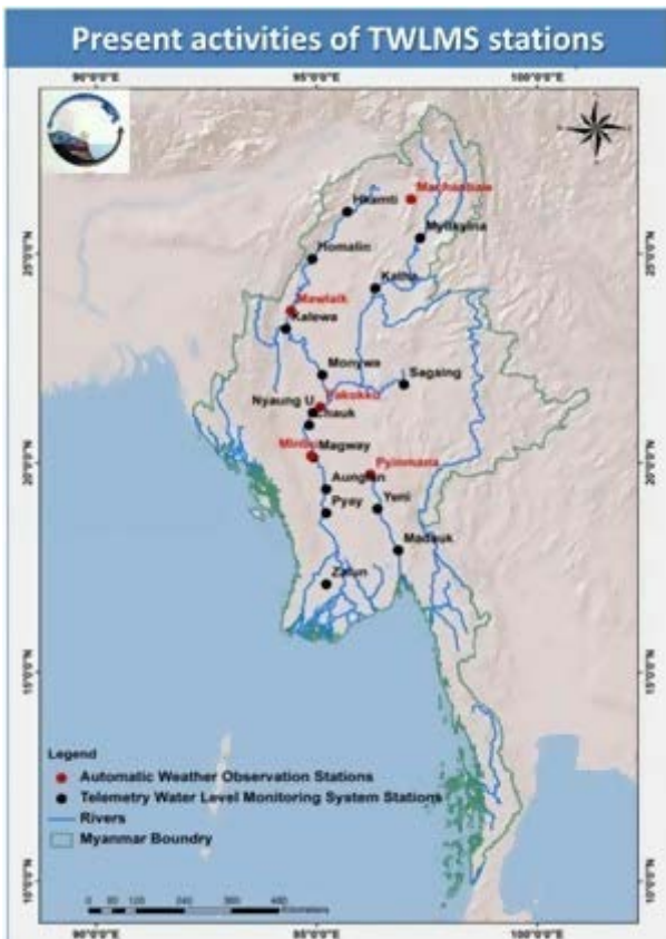
Telemetry water level monitoring system stations in Myanmar
