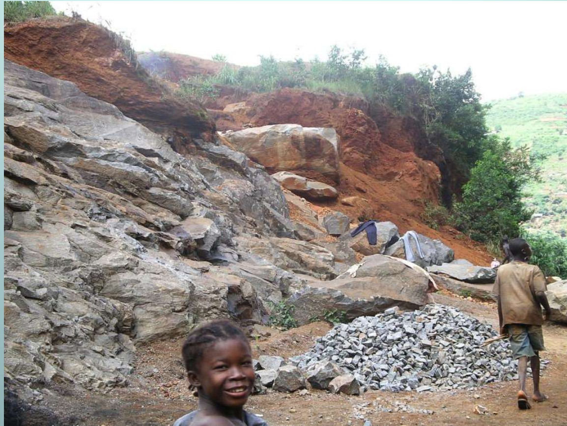
Quarrying of Gabbroic rock for commercialisation of aggregate
